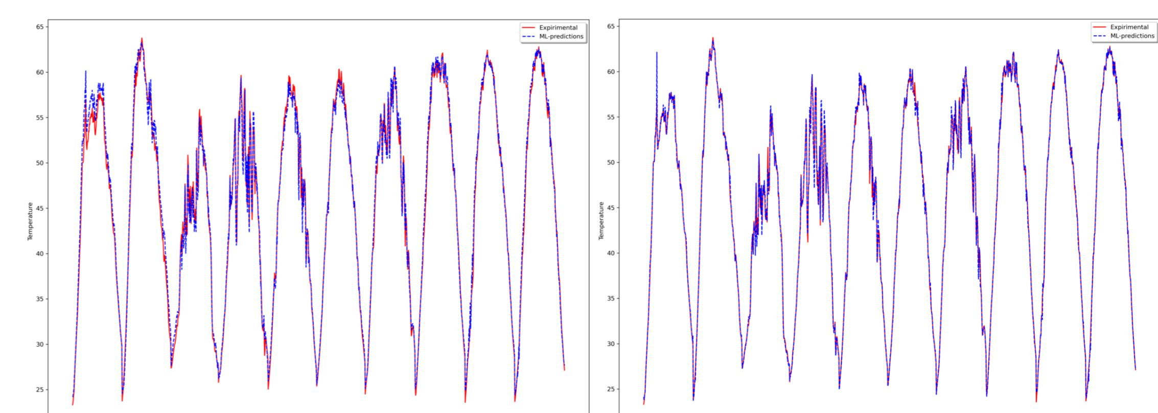
In the figure above we can see the graphs of two different DNNs, comparing the observed temperature (red) with the network's predictions (blue) for the first method. On the left side of the figure we have the predictions of the network with 2 hidden layers and 5 neurons in each hidden layer, while on the right side we have the predictions of the network with 5 hidden layers and 40 neurons in each hidden layer.
