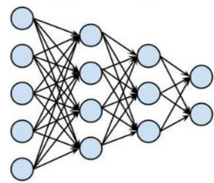
A *feedforward* neural network is an ANN which is described by an algorithm working in layers where the connections between the neurons do not form a cycle and the data are passing from the input neurons to the adjoined neurons and so on.
